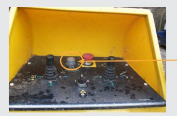
Emergency DC Power button press and hold to activate the electric motor. Use function levers to lower boom sections.
