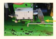
Hand Pump Manifold and Pump Handle Housing
